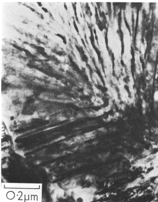
Figure 10 Discontinuous precipitation in splat-cooled Fe-10%Mo-0.5%C aged 1 h at 700°C. Ion-beam thinned foil. Transmission electron micrograph.
