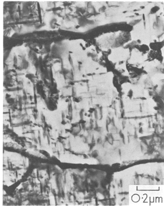
Figure 8 Electropolished foil of splat-cooled Fe-10% Mo-0.5% C aged 20 h at 600^\circ\text{C} , showing the three variants of \text{Mo}_2\text{C} needles within the dendrites of the solidification structure. Transmission electron micrograph.
